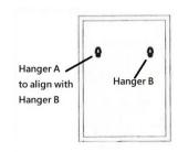
WARNING: Do not use wire between the hangers to hang the mirror from a single screw.
